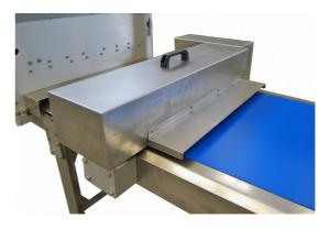
The disc cutter machine can be integrated with a process line; furthermore, the machine is managed from a software and syncronized with the conveyor belt.
